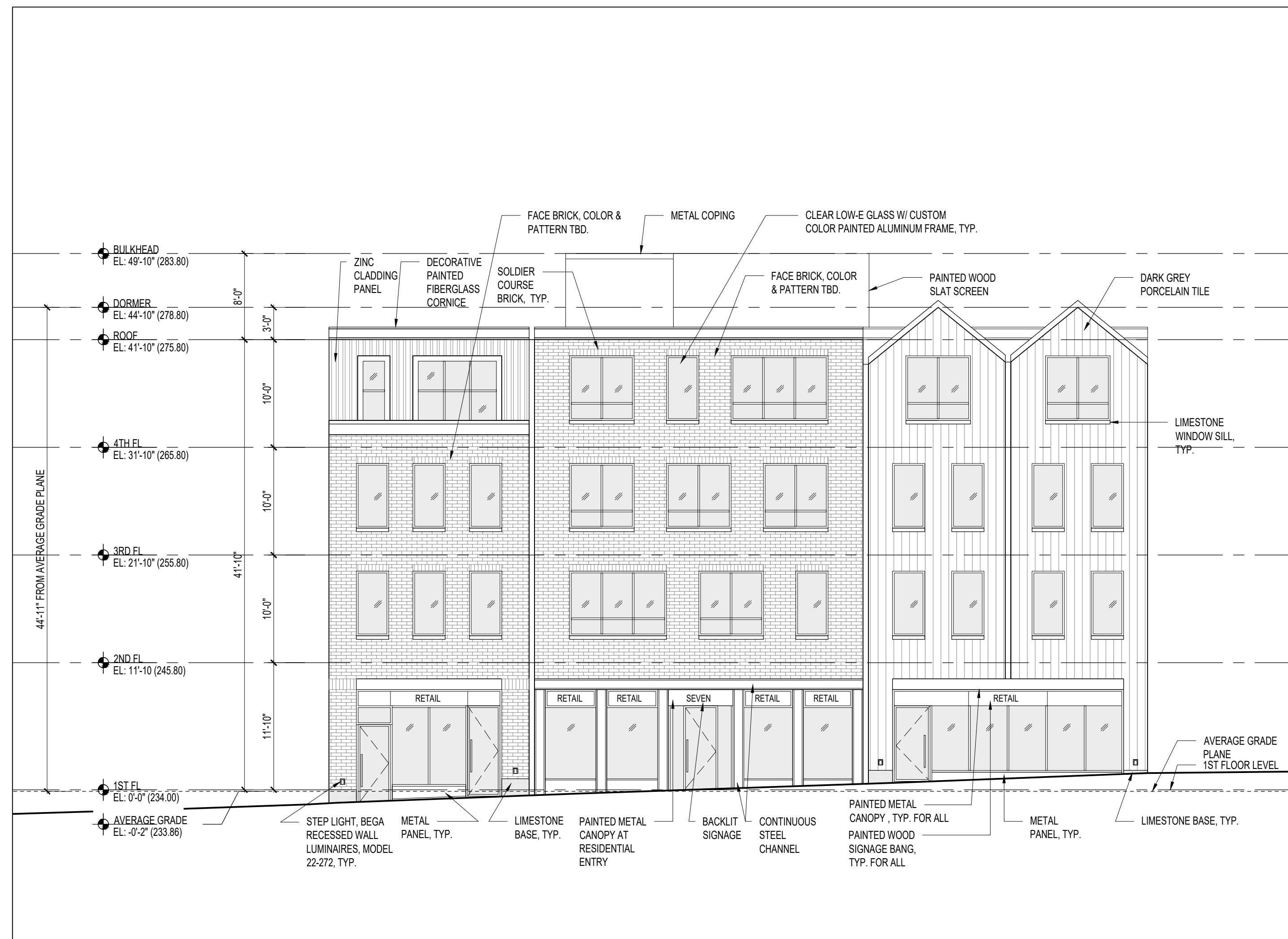
1 | ELEVATION 1 - WEST ELEVATION
